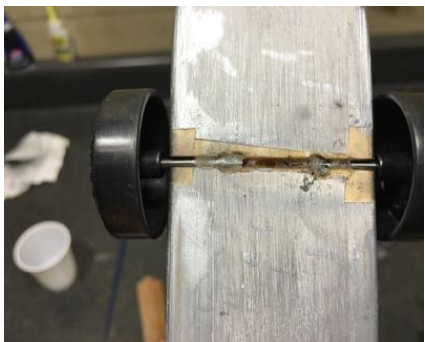
If you are using the pre-drilled axel beds, once your wheels are aligned, fill in the trench with super glue. NOTE: use the super glue gel – sad to say, but that stuff has changed my life!
