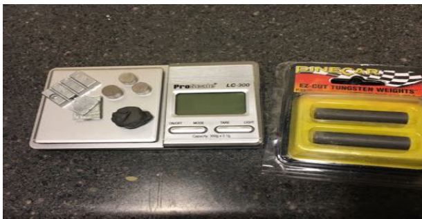
Various weights of various types are available. We like the tungsten putty (on scale, bottom right) and the lead cylinder/tubes (above putty) The tungsten tubes are nice and able to be trimmed, but you get less weight per mass.
